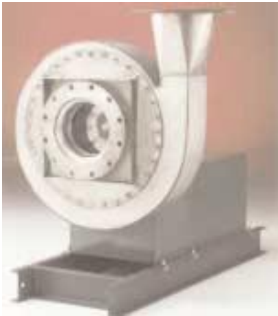
Pressure Blower with stainless-steel airstream and high-build epoxy-coated structure for landfill-methane evacuation.
