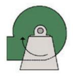
Fan rotation is determined by looking at the fan from the drive end. The drive end is is the side of the fan housing through which the fan or motor shaft protrudes. For DWDI or Arrangement 3 SWSI fans, it is the side of the fan housing at which the belt drive sheave is mounted.
