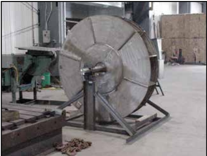
This wheel and shaft assembly was a component replacement in a competitor's fan assembly.
