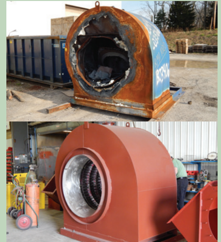
(Above) This is an induced draft fan located on dirty side of baghouse exhausting blast furnace.
