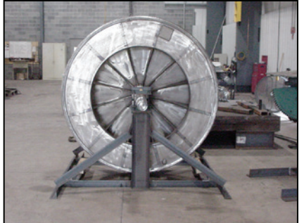
82" radial blade wheel and shaft assembly used on a rotary kiln baghouse in the lime industry.
