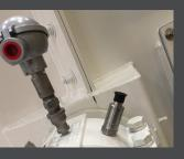
Bearing RTD's (Resistance Temperature Detectors) are used to monitor bearing temperatures. Bearing temperature is a key indicator of bearing health. Identifying temperature increases at the time they occur allows plant maintenance personnel to address potential issues
