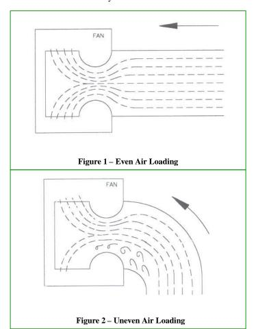
When the system attempts to change the direction of flow, the air hugs the outside of the inlet elbow entering the fan. This causes uneven, turbulent airflow into the fan. Another common cause of non-uniform flow into the fan inlet is a poorly designed inlet box, such as the one shown in Figure 3. It is important to remember that air has mass.
