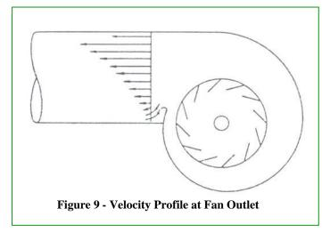
Air is not discharged from a fan with a uniform velocity profile. The main reason for this is the fact that air has weight and is thrown to the outside of the scroll. Figure 9 shows a typical velocity profile.
