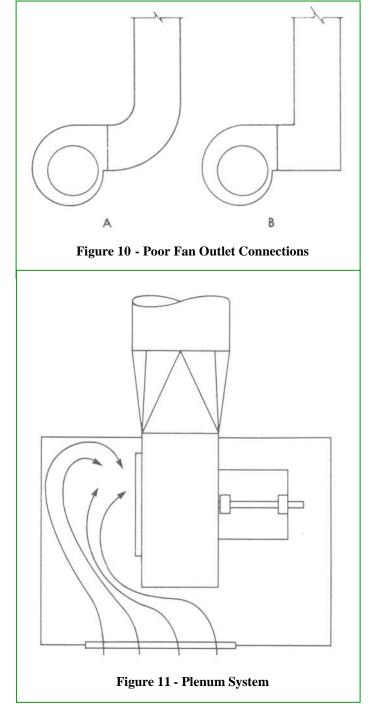
If system effect situations cannot be avoided, their impact on performance should be estimated and added to the calculated system resistance prior to sizing or selecting the fan. Ignoring the system effect could lead to difficult field performance problems later. It could be that the installed fan does not have the necessary speed reserve, or the motor is not of sufficient brake horsepower. The cost of correcting such a field performance problem could escalate rapidly.
