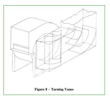
To overcome these losses, the fan speed must be increased to the speed shown in the fan's rating table at the required volume and a pressure 21% greater than originally calculated:
