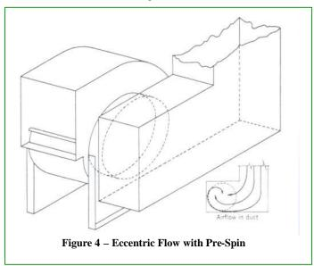
Pre-spinning flow can result from any number of common situations. Two elbows in close proximity to one another can force the air to make consecutive turns in perpendicular planes to form a corkscrew effect. As shown in Figure 5, air converging tangentially into the main duct or plenum can create an obvious spinning effect.
