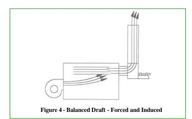
Forced-draft fans and blowers are common for cast iron firetube and small water tube boilers. The fan or blower serves to provide the air and the velocity necessary for the fuel-to-air mixture to enter the actual combustion chamber. When used in conjunction with induced draft, the forced-draft fan is often called the primary air fan since it provides the primary combustion supply air. The induced-draft fan provides the airflow necessary to overcome system resistance and exhaust the flue gases.
