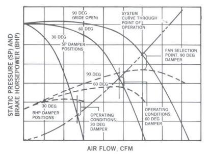
**Figure 2** - Effect of applying inlet dampers to the fan in Figure 1. Separate SP and BHP curves are developed for each vane setting. Fan operating points at these settings are determined by system resistance (points where system curve intersects SP and BHP fan curves).
