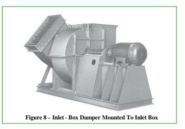
Inlet dampers typically improve the stability of most products because they control the flow through the fan inlet. At extreme dampering, about 30° open, inlet dampers can no longer create a vortex and become essentially a blocking damper. This causes the fan to operate far to the left on its curve. When this happens, a fan is subject to the same problems of instability as if the point of rating was established by an outlet damper or other system changes.
