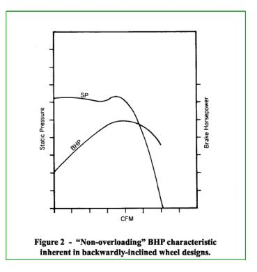
The fan capacity table (Figure 3) shows the fan BHP for a given volume/pressure relationship. However, it is not uncommon to size the motor for a static pressure 5% to 10% higher than design to allow for variances in the installed system. The system designer should also be prepared to reduce fan speed if resistance is lower than anticipated.
