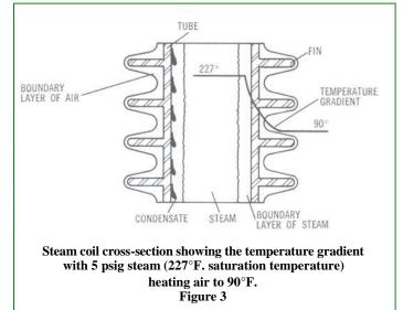
All steam coils are 100% efficient in the sense that the heat released by condensing steam within the coil has nowhere to go but into the air surrounding the coil. Tube-and-fin material, fin spacing, air velocity, and some other factors affect the **rate** at which the heat transfer (and therefore the condensation) takes place but they cannot alter the fact the steam's latent heat has only one place to go: into the airstream.
