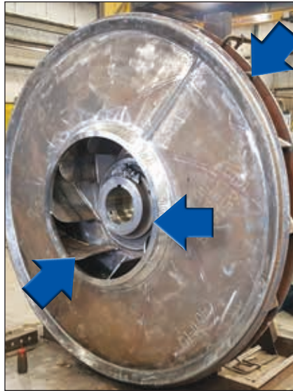
Figure 5: Here are the most common areas to look for cracks in the impeller.
