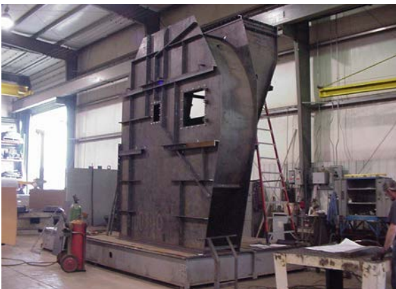
Rugged centrifugal fan housing being constructed.
