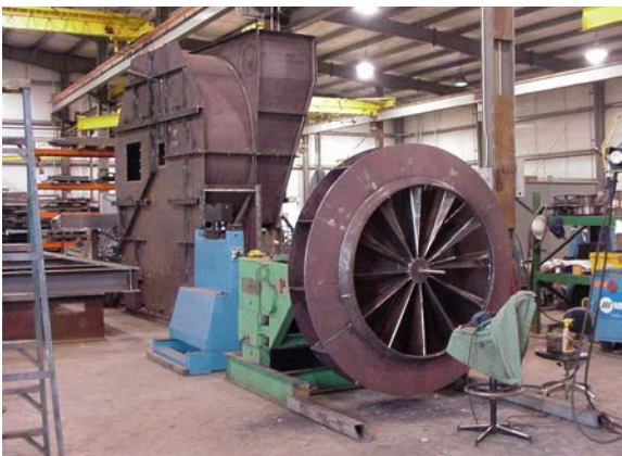
Fan housing and balanced wheel for cement application.
