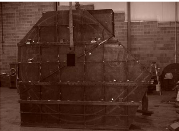
Completed heavy industrial fan for cement production.
