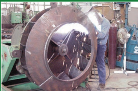
A welder is working on fabricating a New York Blower Company wheel per customer specifications. This flat weld process allows the welder to rotate the wheel so welding is possible at every angle.
