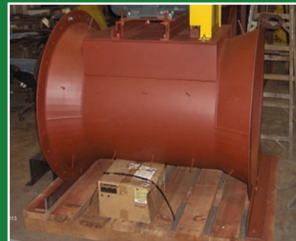
New York Blower Company 700°F Axial Fan used for an industrial furnace exhaust application.
