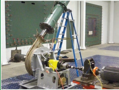
Standard Testing Capacity: New York Blower Company fan being tested for air performance. All testing is in accordance with AMCA guidelines in an AMCA accredited laboratory.
