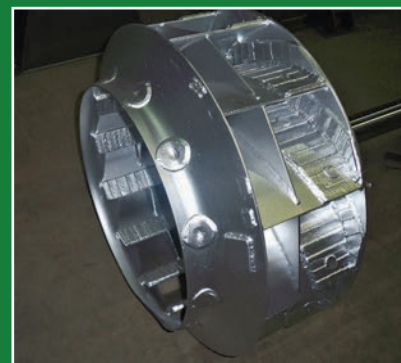
A New York Blower Company repair and rebuild project for a replacement wheel. This duplicate wheel has improved wear performance by adding chromium carbide liners.
