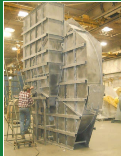
Carbon steel fan designed for a New York Blower Company customer as a repair and rebuild job.
