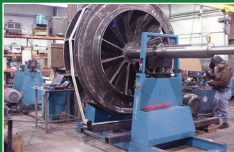
Wheel and Shaft Assembly with Chromium Carbide Liners, SW, 1200 RPM, A514 Steel Construction. Shown being balanced on our large dynamic balancer with a capacity up to 140" diameter and 20,000 lb weight.
