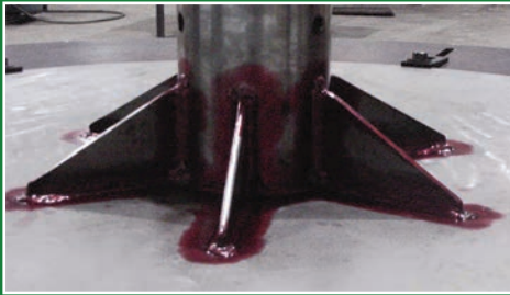
Non-Destructive Testing: Wheel hub being dye penetrant tested per AWS D14.6. Other test methods available include magnetic particle, X-ray and ultrasound. NDT inspection is done by New York Blower Company and independent third party inspectors as required by customer.
