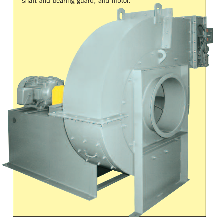
Size 364 Arrangement 8 Series 30 GI Fan with flush-bolted cleanout door, split housing, external outlet damper, coupling guard, shaft and bearing guard, and motor.
